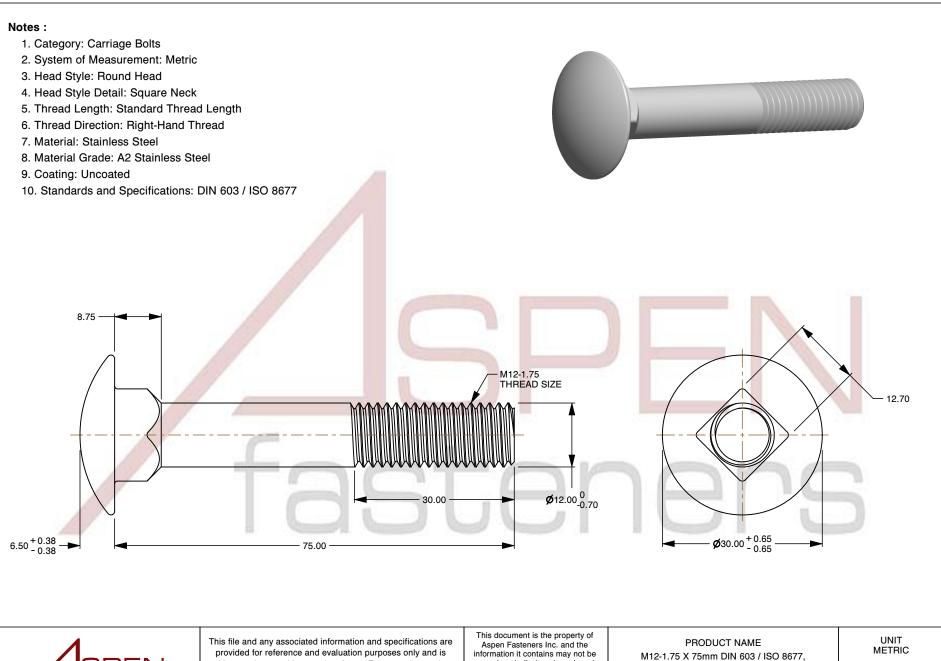
fasteners www.aspenfasteners.com This file and any associated information and specifications are provided for reference and evaluation purposes only and is subject to change without notice. Aspen Fasteners Inc. makes no representations, warranties, or guarantees as to the appropriateness, accuracy, completeness, or suitability for any purpose of the file, information or specifications. You are solely responsible for the use of the file, information, or specifications.
