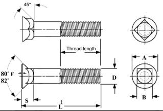
‡Length of a plow bolt is measured from the top of the head to the extreme end of the bolt.
